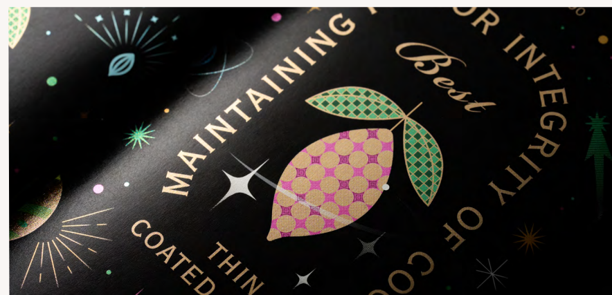
Sheet-fed Offset Cold Transfer – Thin Paper Packaging Application
